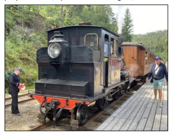
locomotives were rescued and have now been brought back into use. The original locos, 2-4-2T, supplied were by Dubs and we had locomotive no 5. a copy of the earlier locos, which was built in Norway.
