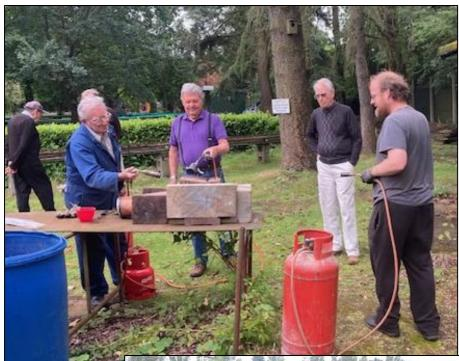
On the 27<sup>th</sup> July at the track, we had Dave being helped to apply enough heat to repair a leak which was found on the foundation ring on his boiler.
